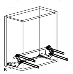
Step 2. Attach the lifting rods (A,B) to the left and right base brackets (D-L,D-R) as shown.
