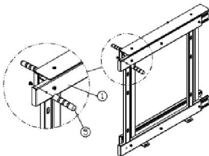
Step5: Install plastic hooks as shown.
