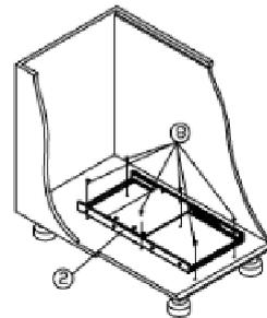
Step4: Loosen the hexagon socket screw on the base frame, install the main frame on the base frame and lock the screw as shown in the picture.
