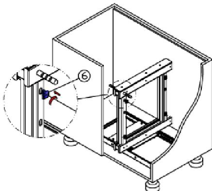
Step2: The base frame is aligned with the fixed mounting hole on the base plate and is screwed tight.
