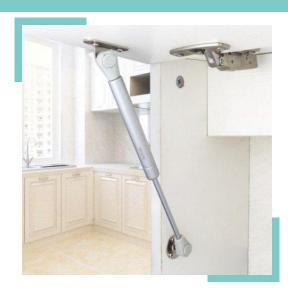
pressure difference between the cylinder and external atmospheric pressure acting on the cross-section of the piston rod. High-pressure inert gas powers the support rod and ensures a stable support force throughout the working stroke. A buffer mechanism can prevent the cabinet door or lid from slamming when we close the door. The constant gas pressure inside the cylinder and the fixed cross-section of the piston rod make the force of the support rod stable throughout the stroke.
