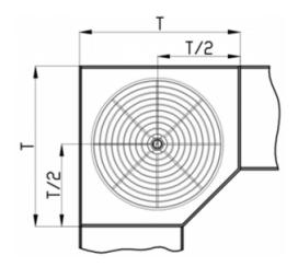
Step 1: Draw two auxiliary circles on the top and bottom plates as shown.
