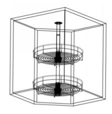
Step 4: Fix the top and bottom of the tube Step 5: Adjust the height of the basket to a proper position with the bolt and tighten the plastic parts.
