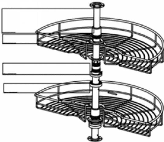
Step 4: Fix the top and bottom of the tube to base with eight ST3.5\*16 screws.
