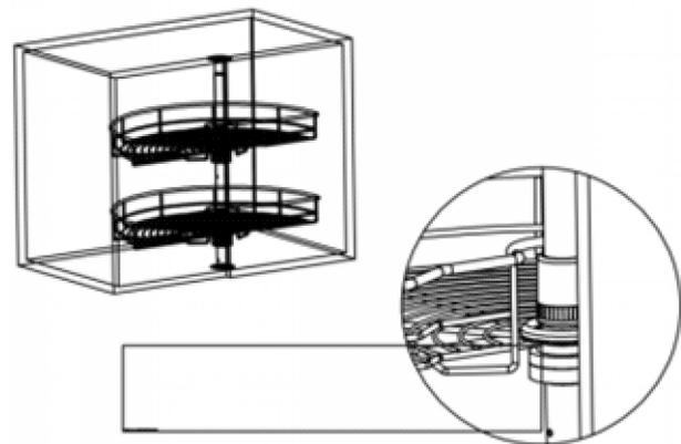
Step 5: Adjust the height of the basket to a proper position with the bolt and tighten the plastic parts.
