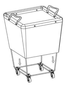
Step 5: Fix the top frame to the bracket with screws.
