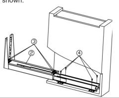
Step 3: Mark the mounting holes on the cabinet door as shown.
