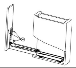
Step 5: Install the organizer frame on the base frame as shown.
