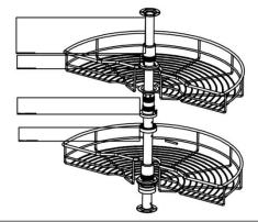
Step 4: Fix the top and bottom of the tube base with eight ST3.5\*16 screws.
