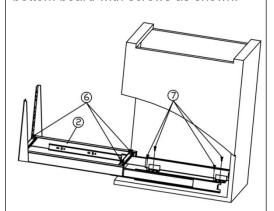
Step 3: Mark the mounting holes on the cabinet door as shown.
