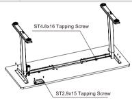
Desk Tops made by Hi5 are reserved with mounting holes on the backside. Please adjust the width of the desk frame according to the position of the mounting holes.
