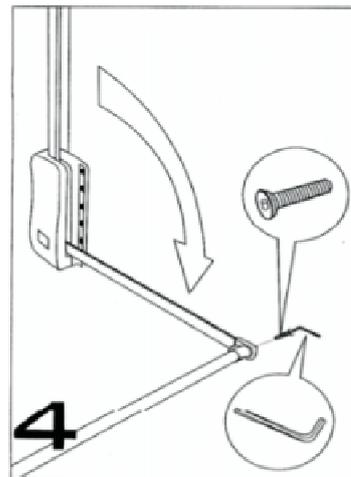
Step 5: Adjust the width of the hanging rod to a proper position, and then tighten it clockwise.
