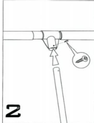
Step 3: Fix the handle on the wardrobe rod by using M3 screws. Adjust the length of the hanging rod to be less than the width of the closet by 9 cm.
