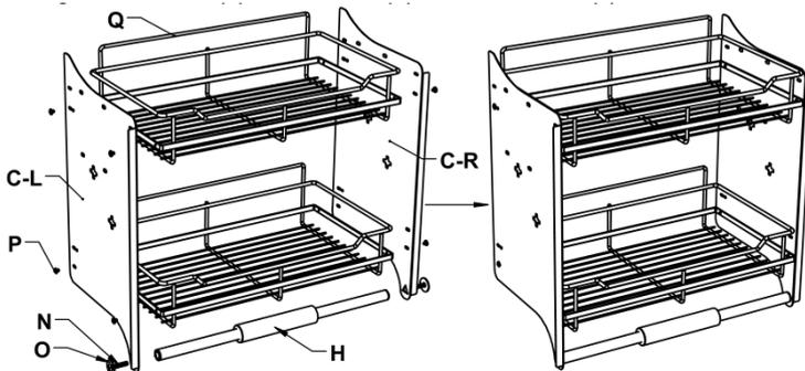
Step 5. Mount the assembly 9stem 4) to the base brackets (step3) using 4 axle sleeves (J), 8 M6\*12 screws (L) and 8 flat washers (O) as shown.
