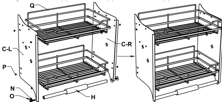
Step 5. Mount the assembly 9stem 4) to the base brackets (step3) using 4 axle sleeves (J), 8 M6\*12 screws (L) and 8 flat washers (O) as shown.
