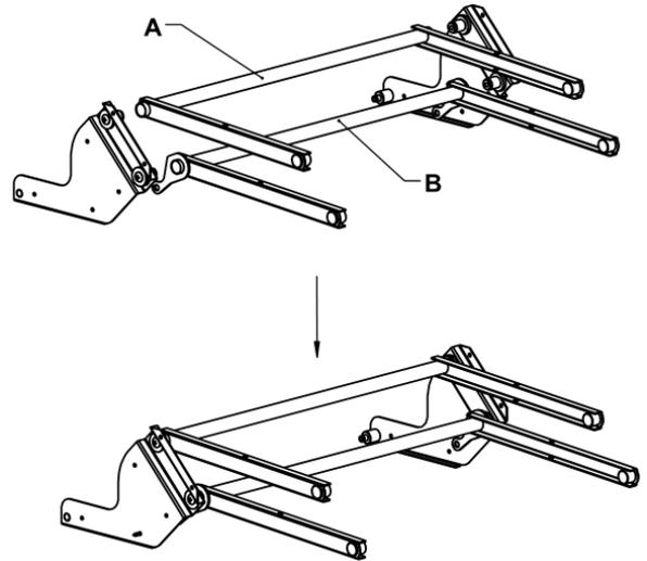
Step 3. Mount the assembled base brackets (step 2) to the side panel of the cabinet using 12 ST4.0\*16 SCREWS (k) as shown.
