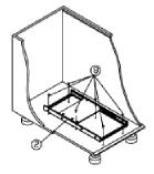
Step4: Loosen the hexagon socket screw on the base frame, install the main frame on the base frame and lock the screw as shown in the picture.
