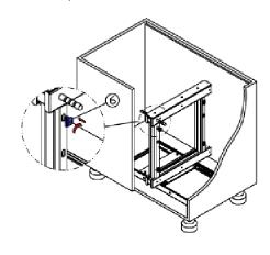
Step2: The base frame is aligned with the fixed mounting hole on the base plate and is screwed tight.
