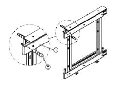
Step5: Install plastic hooks as shown.
