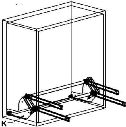
Step 4. Attach two wire baskets (Q) and the handle (H) to the side panels (C-L,C-R) using 2 M6\*30 screws (N), 2 flat washers (O) and 8 M4\*5 screws (P) as shown.
