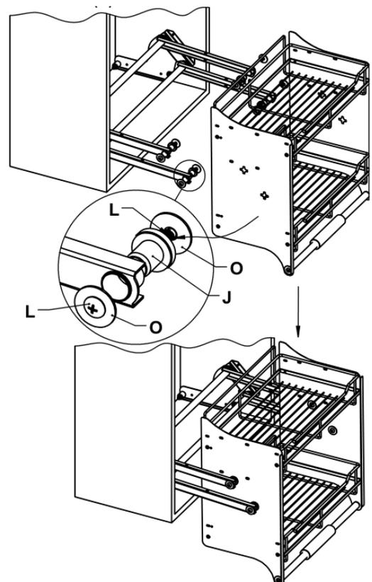
Step 6. Mount 2 pneumatic rods (E) to the base brackets (D-L,D-R) using
