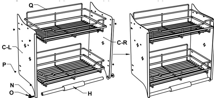
Step 5. Mount the assembly (step 4) to the base brackets (step 3) using 4 axle sleeves (J), 8 M6\*12 screws (L) and 8 flat washers (O) as shown.
