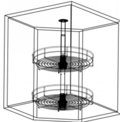
Step 4: Fix the top and bottom of the tube to base with ten ST3.5\*16 screws.
