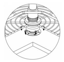
Step 1: Draw two auxiliary circles on the top and bottom plates as shown.
