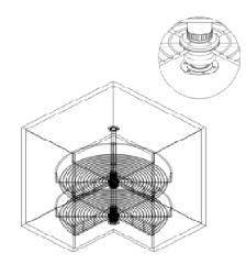
Step 4: Fix the top and bottom of the tube Step 5: Adjust the height of the basket to a proper position with the bolt and tighten the plastic parts.
