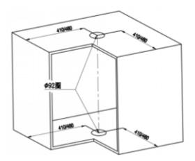
Step 3: Place the basket in the cabinet based on the auxiliary center point and adjust the angle of the basket.
