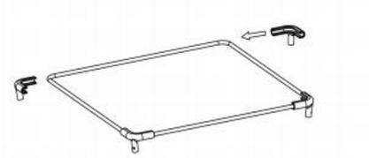
Step 4: Connect the assembled top frame to the brackets.
