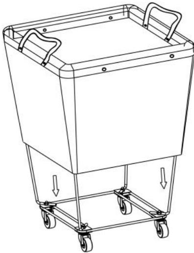
Step 5: Fix the top frame to the bracket with screws.
