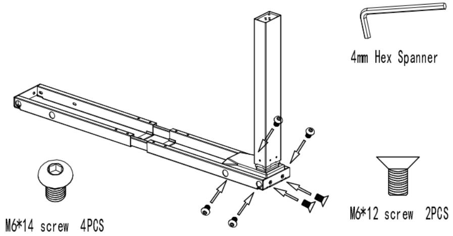
**6** Attach feet to the legs using 4 of M6\*14 screws, attach the 2 of levelling foot pads to the feet by hand
