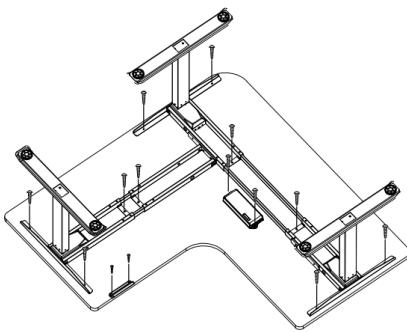
**10** Connect the control box to the handset and to the motor
