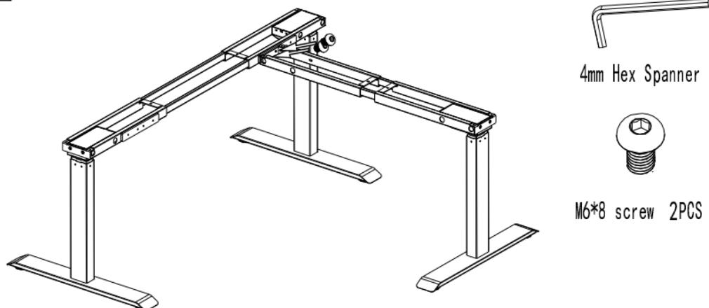
**8** Attach brackets to beam using 6 of M6\*12 screws, and then fit the rubber cushions to the brackets and beams
