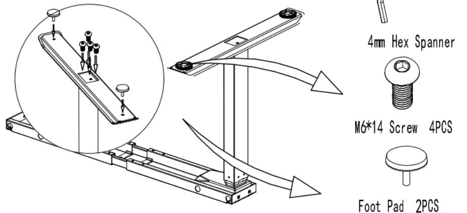
**7** Attach the beam2 to the beam1 using 2 of M6\*8 screws
