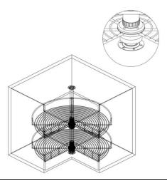
Step 5: Adjust the height of the basket to a proper position with the bolt and tighten the plastic parts.
