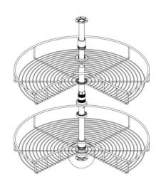
Step 4: Fix the top and bottom of the tube base with ten ST3.5\*16 screws.
