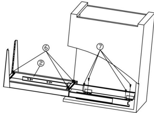
Step 3: Mark the mounting holes on the cabinet door as shown.
