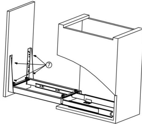
Step 5: Install the organizer frame on the base frame as shown. And install other accessories on the corresponding positions of the organizer frame.
